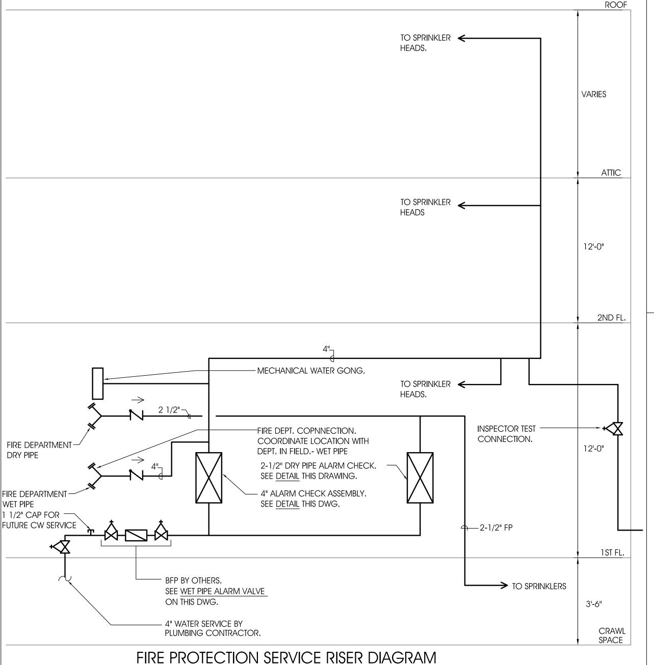
1. PIPE SIZES PROVIDED FOR BID PURPOSES. ALL PIPE SIZES TO BE PER HYDRAULIC CALCULATIONS. SEE SPRINKLER SYSTEM
